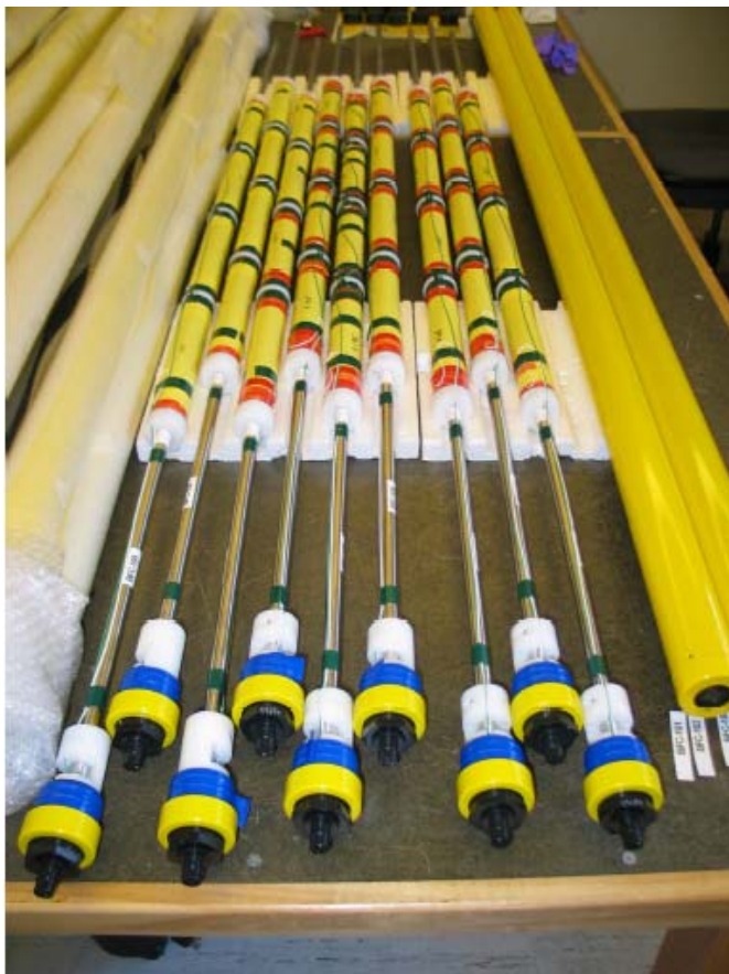
Figure 18. Magnetic induction coils during the manufacturing process at SIO (photo courtesy of Scripps Institution of Oceanography).
